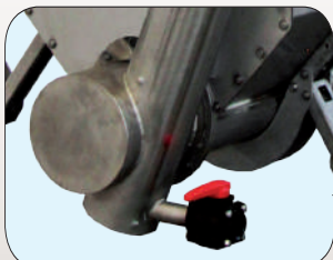
Extracting screw with variable inclination
