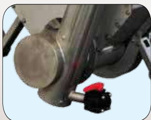
Extracting screw with variable inclination
